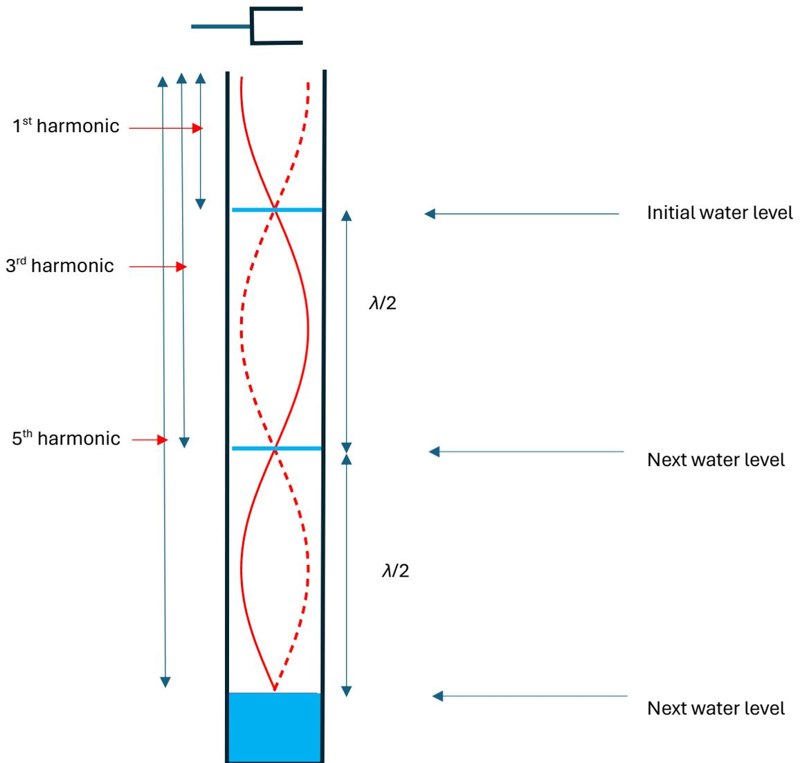
The horizontal lines show the level of the water for each harmonic. It is clear from the diagram that the water level has to be lowered by a distance equal to half a wavelength to get the next harmonic.
